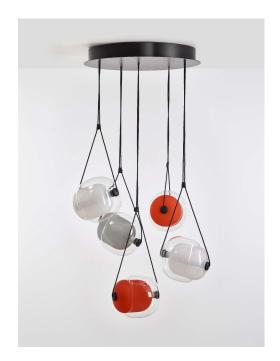
**Tech. description** Capsula comprises three glass components. The light source is housed in a glass tube and uses special Brokis connectors in metal end caps. The end caps hold the light together even once the cords have been removed. The light is hung from a ceiling canopy, which also contains the electronics.
