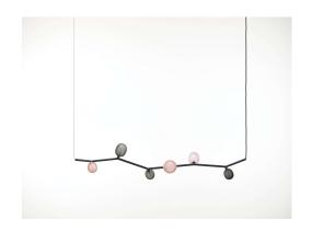
**Tech. description** The main body of the light comprises a dural frame and glass shades fitted with G4 sockets. The frame is connected to the power cable by means of an integrated Brokis connector and is hung from a steel rope on the opposite end. The power cable is hung from the ceiling canopy, which also houses the electronics.
