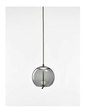
Tech. description The light comprises a glass shade, glass diffuser, metal component with LED module, and linen rope and is suspended from the ceiling canopy with a special bracket. The bottom section of the light is engineered as SELV.
