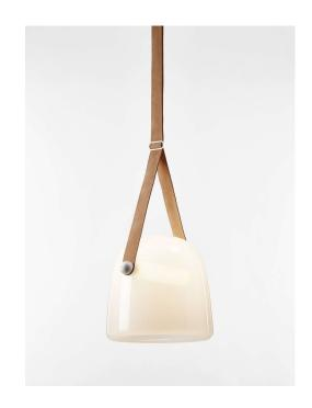
Tech. description The light comprises a glass shade, leather suspension straps, and tubular LED module with triplex opal glass diffusor. The LED module uses a Brokis connector. The entire assembly is secured with dural endcaps. The light is hung from a ceiling canopy, which also houses the electronics and terminal connectors.
