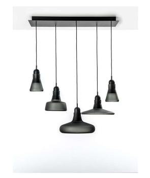
Tech. description The light consists of a wooden body with connector and E27 light source socket. It also includes a lead cable with connector, the glass shade, and a wood ceiling canopy.
